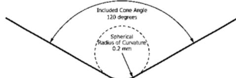
**FIG. A3.1 Diagram of Cross-Sectional View of Spheroconical Diamond Indenter Tip**
