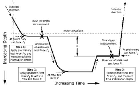
FIG. 1 Rockwell Hardness Test Method (Schematic Diagram)
