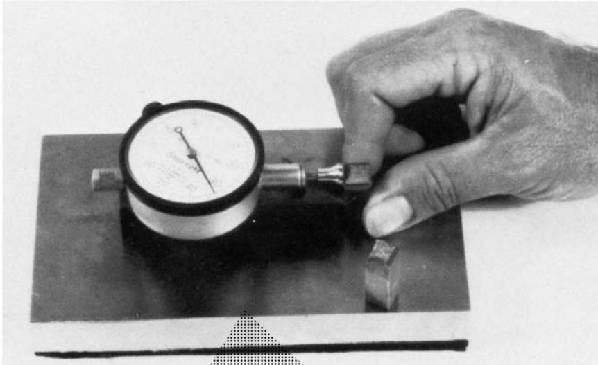
FIG. 16 Lateral Expansion Gauge for Charpy Impact Specimens
